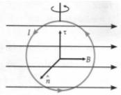
In Fig. n is a unit vector normal to the plane of the loop, directed outward. The angle between n and B is 90°. The magnitude of the torque acting on the loop is
