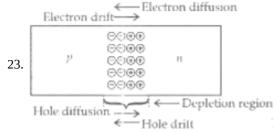
Due to the diffusion of electrons and holes, from their majority to minority zone, a layer of positive and negative space charge region on either side on the junction is formed. This is called the depletion region. The loss of electrons, from the n-region and the gain of electrons by the p-region, cause a difference of potential across the junction formed. This tends to prevent the further movement of charge carriers across the junction and is, therefore, termed as barrier potential.
