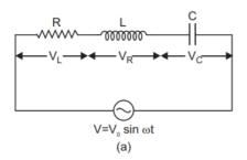
Suppose the voltage across resistance R is  $V_R$ , voltage across inductance L is  $V_L$  and voltage across capacitance C is  $V_C$ . The voltage  $V_R$  and current i are in the same phase, the voltage  $V_L$  will lead the current by angle  $90^o$  while the voltage  $V_C$  will lag behind the current by angle  $90^o$ . Clearly  $V_C$  and  $V_L$  are in opposite directions, therefore their resultant potential difference =  $V_C$  -  $V_L$  (if  $V_C > V_L$ ).
