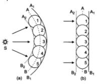
The Huygens' construction gives a backward wavefront also shown by dotted line A2B2 which is contrary to observation. The difficulty is removed by assuming that the intensity of the spherical wavelets is not uniform in all directions; but varies continuously from a maximum in the forward direction to a minimum of zero in the backward direction.
