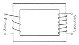
Input power,  $P_i$  =  $I_i \times V_i$  = 15  $\times$  100 = 1500 W
